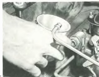
Checking Fuel Flow
