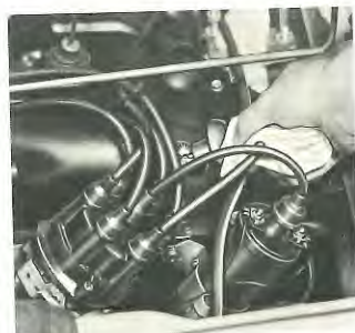
Checking for Spark
