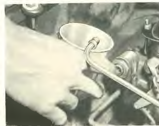
Checking Fuel Flow
