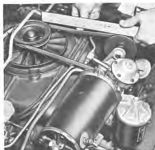
Checking Fan Belt Tension
