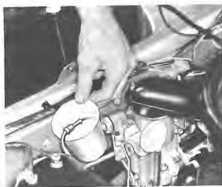
Checking Fuel Flow
