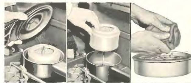
REMOVAL AND CLEANING OF ELEMENT
