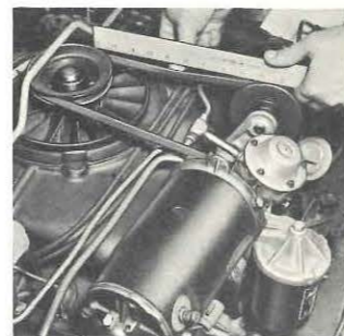
Checking Fan Belt Tension
