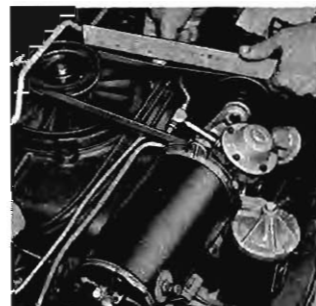
Checking Fan Belt Tension
