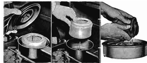
REMOVAL AND CLEANING OF ELEMENT
