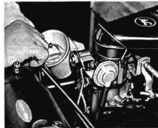
Checking Fuel Flow
