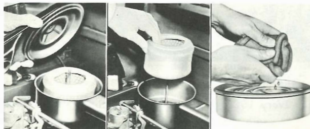
REMOVAL AND CLEANING OF ELEMENT
