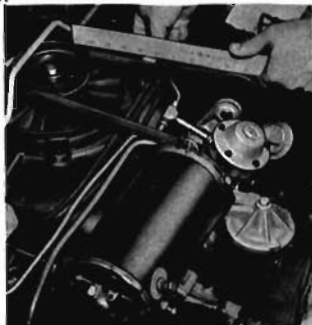
Checking Fan Belt Tension
