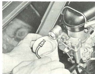
Checking Fuel Flow
