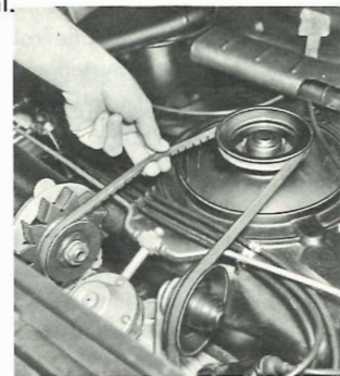
Checking Fan Belt Tension
