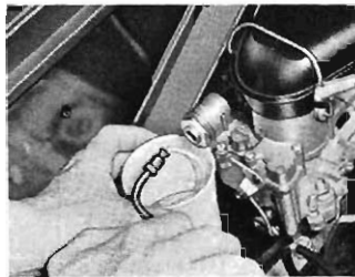
Checking Fuel Flow
