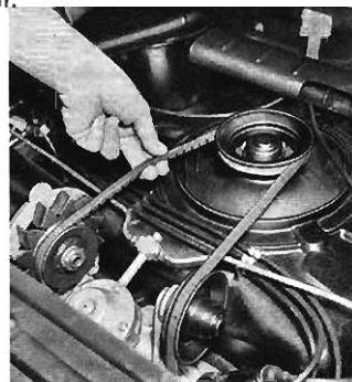
Checking Fan Belt Tension
