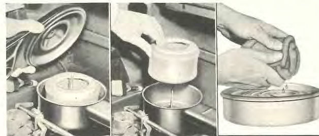
REMOVAL AND CLEANING OF ELEMENT
