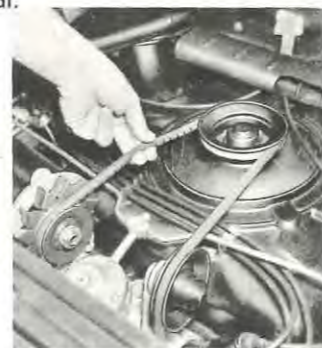
Checking Fan Belt Tension
