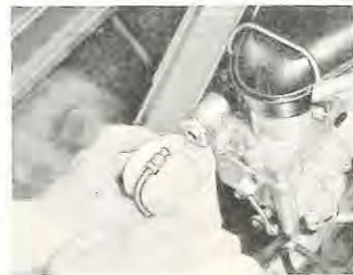
Checking Fuel Flow
