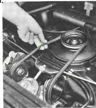
Checking Fan Belt Tension
