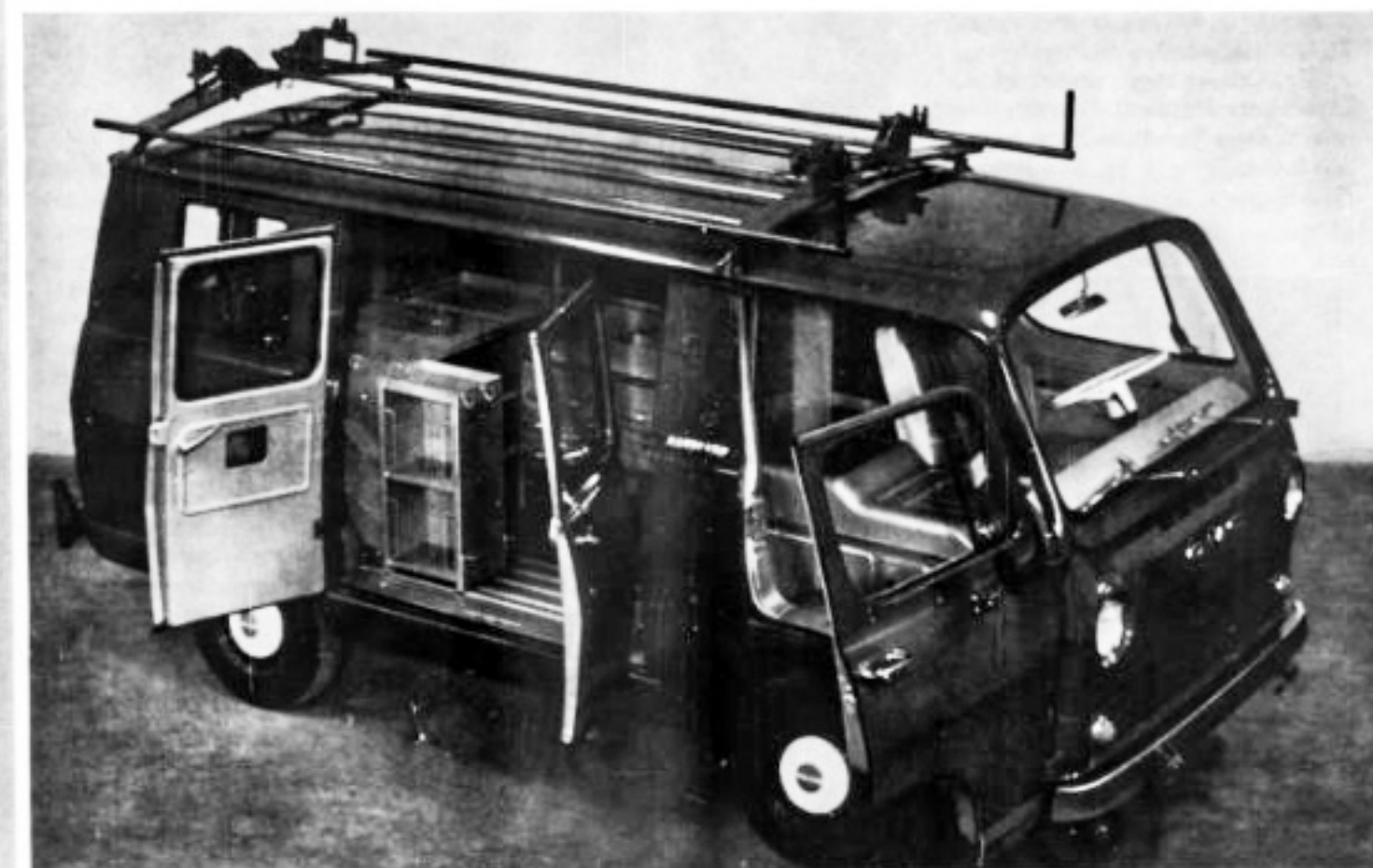
There are more than 15,000 of these compact vans in Bell System service today. The ladder brackets on the top of the van and much of the interior compartmentation were designed specifically by Bell Laboratories.
