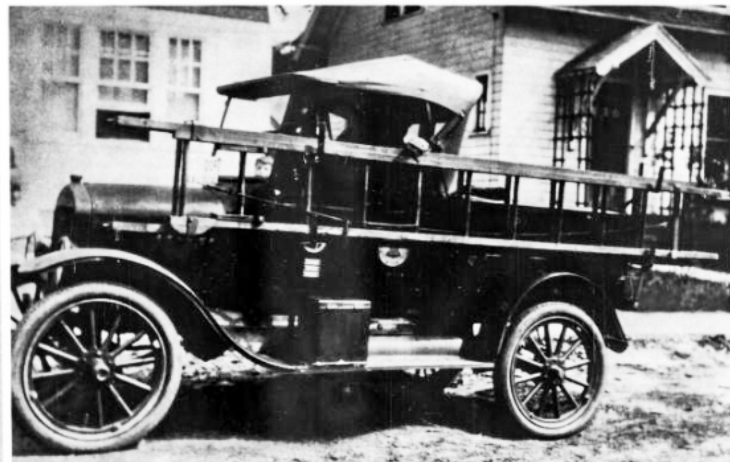
This was the transportation available (sometimes) to the telephone installation craftsman of yesterday. The photograph was taken about 1916. Note the Bell System seal on the side panel of this MODEL T runabout.
