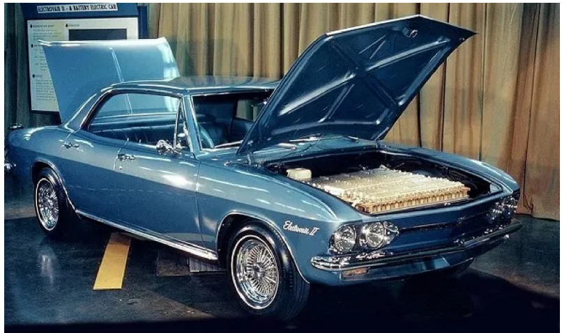
General Motors has a long and varied history with alternative-fuel vehicles. Here's an interesting example from 1966, the battery-electric Electrovair II.
