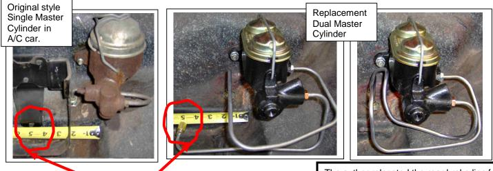
Both the Clark's Corvair and Corvair Underground kits are not compatible with Air Conditioned cars. Bending the rear brake line inside the car is also required. The author relocated the rear brake line from the master cylinder to clear the windshield washer bracket. The new location DOES NOT require any bending of the <u>rear brake</u> <u>line inside the car.</u>
