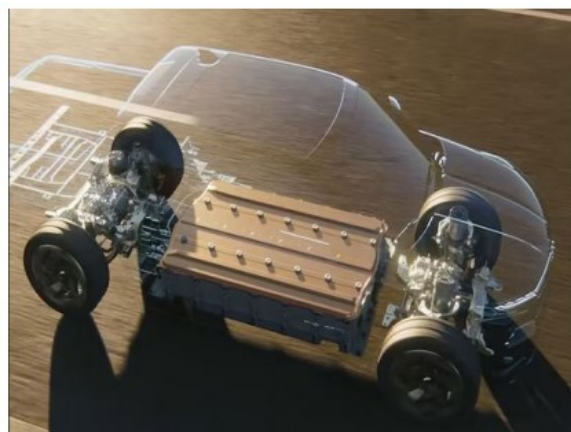
Figure 3: Ultium battery in Silverado EV
