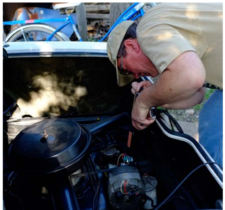
RIGHT: Ned was checking the total advance on his white coupe. Many tune-ups were performed at this Juna Tuna at the Kalp Shop.
