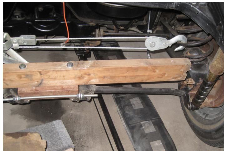
This photo shows how the 2x4 fits on the trailing arm and how the come-along hooks to the springs.
