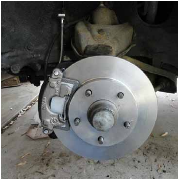
Ned's latest project on his LM white Monza coupe was a disc brake conversion for the front. The caliper brackets were picked up in Indy and the rest of the parts locally.
