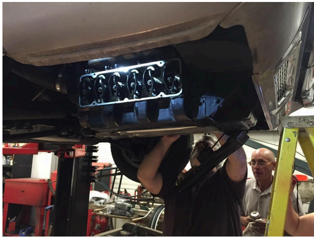
Left - Scott Olivier adjusts rocker nuts during a tech session in 2016 while Dave Dykwell looks on, Right - Ryan Counterman on the ladder turning the crank while Dan Konkle and Dennis Willson adjust the rocker nuts in 2018
