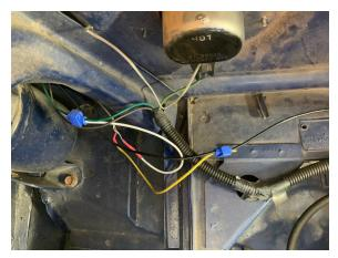
Found some leftover trailer wire and soldered to the led leads (red shrink tubing). The lights are polarity sensitive, so check for that. Took the opportunity to add the black wire as a soldered ground to the light sockets.
