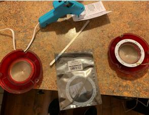
Aluminum flashing cut in strips (4" length x  $\frac{1}{4}$ "wide); hot glued in place; acts as a spacer to the lens and blocks light to the center reverse bulb.
