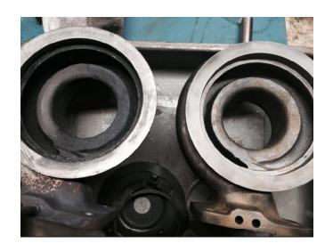
Ended up not being the greatest idea, but I took a thou or 2 off the exhaust seal ID for a nice smooth sealing surface. This ended up opening the overlapping seal ring more than intended. More on that later, but probably the best method would be to take a brake hone and clean it up that way.
