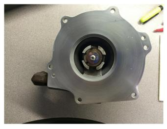
The housing on the impeller side loves seeing the face of a roto-polisher. Muy bueno! Pic is about half way done with it. 320 grit worked well. Took 2 thou to get all the scratches off. Important to have as smooth a surface as possible through the turbo (rough surface = more pressure drop = bad, mmmk.)
