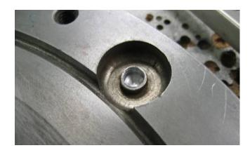
**Step 4:** Get out the 5/16" drill and drill down into the 1/4" hole. You won't need to go down far, just enough to shear off the head.
