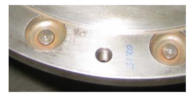
**Step 3:** Drill a 1/4" hole into the rivet about the height of the rivet head.
