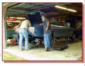
Dan's experience paid off in getting the powertrain to go in the car smoothly. First we raised the front back to its original level. Then we raised the motor until we could loosely install the three bolts that hold the transmission to the front cross member. That done, we bolted in the
