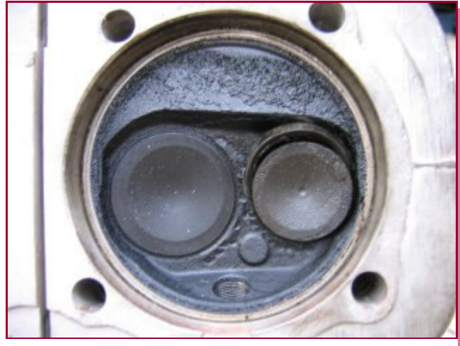
A close up of Dave Ziebarth's cylinder head showing the dropped seat.
