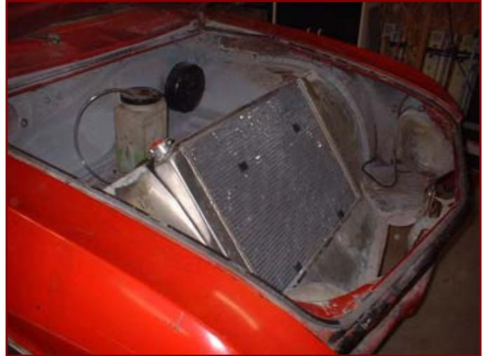
ing to look once complete. Also he showed the modifications that were made to the trunk to accommodate the radiator and the new power brake booster.
