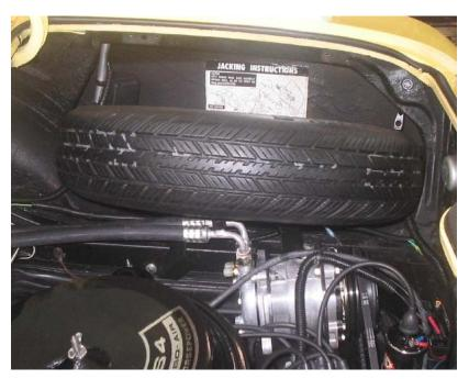
The last photo shows that little radial compressor at the back of the engine, nestling discreetly beneath a spare tire from the trunk of some water pumper, keeping Cecil and his passengers cool and dry as they cruise through the steamy heat of Florida's Space Coast.
