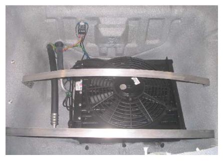
The unit is a Danhard integrated condenser with fan and baffle rated at 21KBtu per hour. It draws air through two slots in the front of the trunk tub, and blows it out straight down. The shiny horizontal bands are supports for an attractive cover Cecil keeps over the rig when he isn't photographing it.
