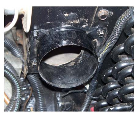
so that he could attach a(n extra) hose connector from the cool-air intake of the heater found at the front of the engine's top shroud. This connector, which attaches very simply with three screws, calls for 3-inch air hose, which Wade attached with the usual clamp and routed to the air cleaner.
