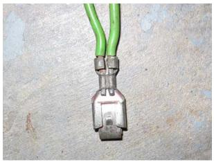
12-gauge wire are crimped into one terminal. For these positions (see drawing), a different terminal is recommended:
